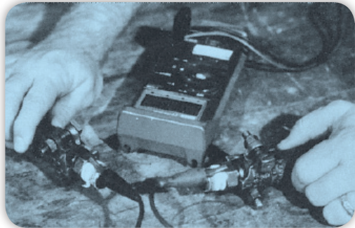
Hose assembly being tested with ohmmeter.
