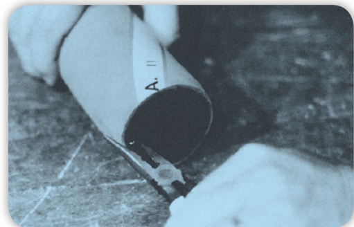
Pinching the staple into the tube wall.
